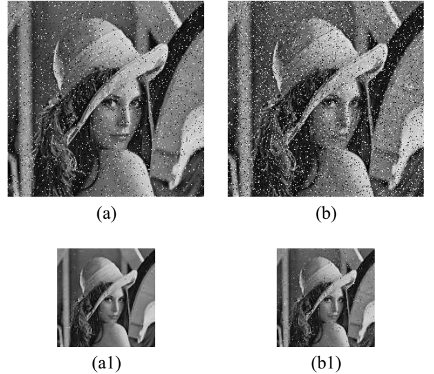
Fig. 8. Reduction of image Lena with noise using the median operator with block sizes of 2 \times 2 .
